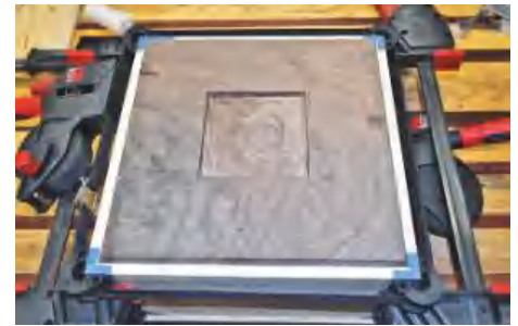
▲ Pic.6 Once the sides and walnut top were clamped together, I let it sit so the glue would dry overnight. But again, no glue was touching the walnut, just the four sides
